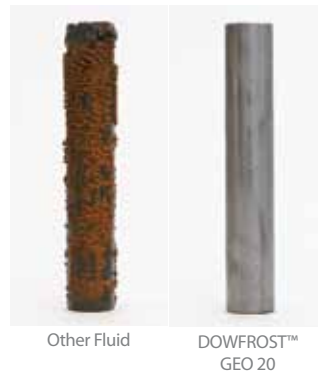
Figure 2 - Two-year Corrosion Comparison
