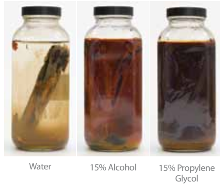
Figure 1 - Alcohols and Improperly Inhibited PG Pose a Corrosion Threat
